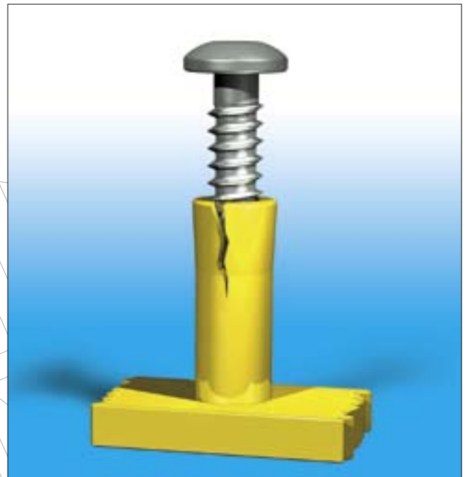
Figure 50 A boss split due to using lubricants to ease insertion.
